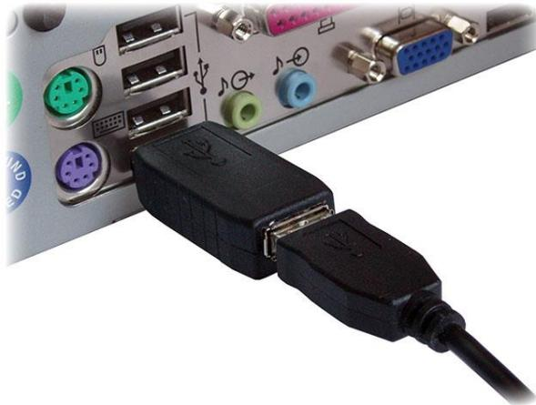
**To view recorded data**, plug the device in-between the keyboard and USB port, and press the 3-key combination **simultaneously** (by default K, B, S)
