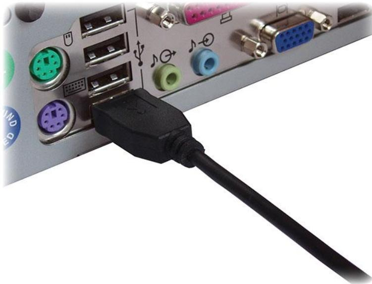
**Disconnect the USB keyboard from the USB port at the computer or hub.
