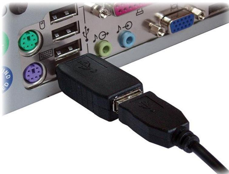
**Connect the hardware USB keylogger between the USB keyboard and the USB port.
